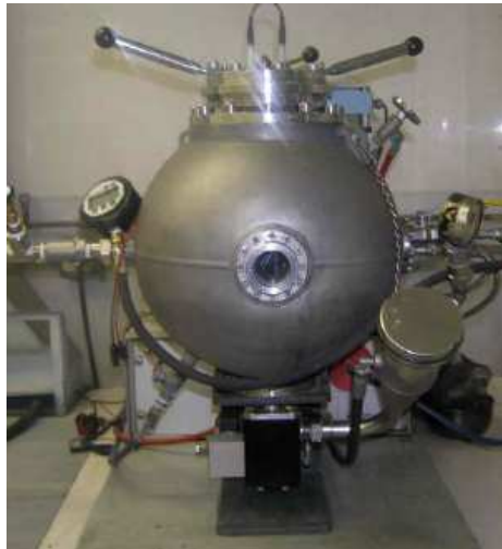
20-liter test vessel for explosivity testing
